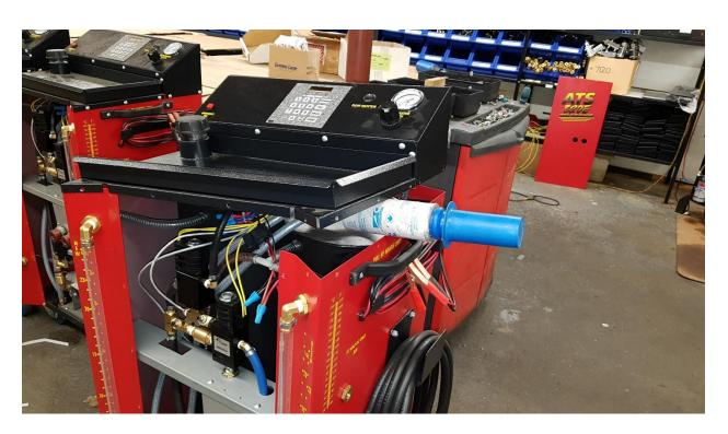
2. To install the new needle valve #7121. Looking at the top of the ATS "Used Fluid Tank". Remove the current hose in place and turn the existing brass fitting already in the used tank, so it at a 90-degree angle. Then attach the open-end hose of the #7121 and clamp the hose. Look at next picture for more details.
